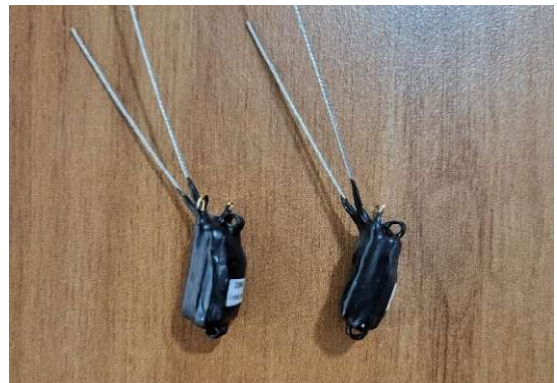
Figure 6. Tags 208603 and 208608 were decommissioned in 2023 due to battery failure/expansion. Not to scale.
