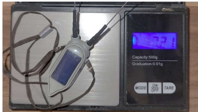
Figure 2. Weight (7.21 g) of a Golden Plover satellite tag (PP-ARG-SOL-40) including harness and breast-loop crimp. Source: WBRU (2022).
