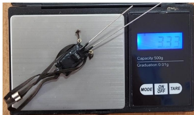
Figure 4. Weight (3.33g) of a Song Thrush satellite tag (PP-ARG-40 light) including harness and breast-loop crimp. Source: WBRU (2022).
