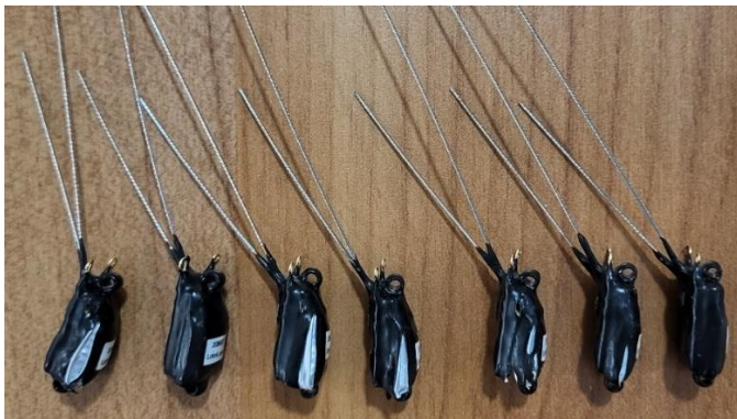
Figure 5. Seven Song Thrush tags were decommissioned in 2022 (note damage to black potting due to battery expansion). Not to scale.
